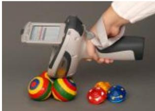
Bay County Health Department's Environmental Health Division purchased an XRF (X-ray Fluorescence) Niton Lead Analyzer in 2009. X-Ray Fluorescence is a non-destructive method of testing for lead content. It has been used successfully for measuring lead in soil and paint, including paint on children's toys, furniture, and other objects. This program will be available in year 2010. More details to follow.
